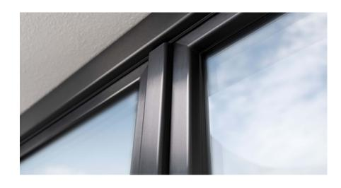
GEALAN-acrylcolor profiles have been manufactured using the co-extrusion process since 1980. GEALAN sets a benchmark with this surface technology, because it differs significantly from typical coloring processes. During co-extrusion, the uPVC base body and the high-quality acrylic glass layer are inseparably bonded together.
